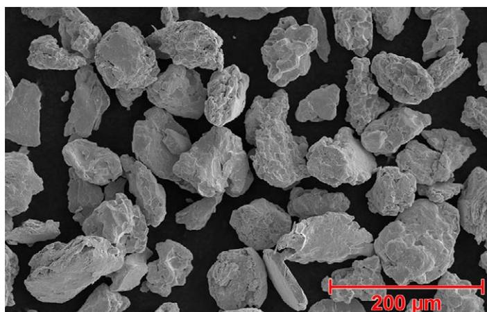
SEM photomicrographs: Top: Metco 4063 (agglomerated and sintered); bottom Metco 63NS (sintered and crushed).
