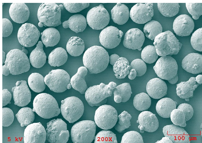
SEM photomicrographs of Metco 58NS, showing morphology that is typical for these products.
